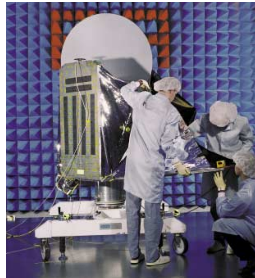
Odin at EMC-test. Credit: Saab Ericsson Space.
